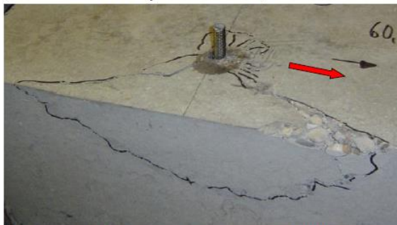
(b) n = 1, M16, h_{ef} = 80 \text{ mm}, c_{l,1} = 100 \text{ mm}
