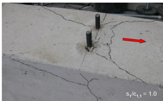
(a) n = 2, M16, h_{ef} = 80 \text{ mm}, c_{l,1} = 100 \text{ mm}
