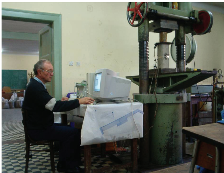
Fig. 7 Testing equipment for monitoring and acquisition of stress-strain data
