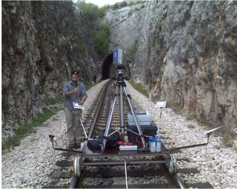
Figure 4: The cart with installed arms with circular targets.
