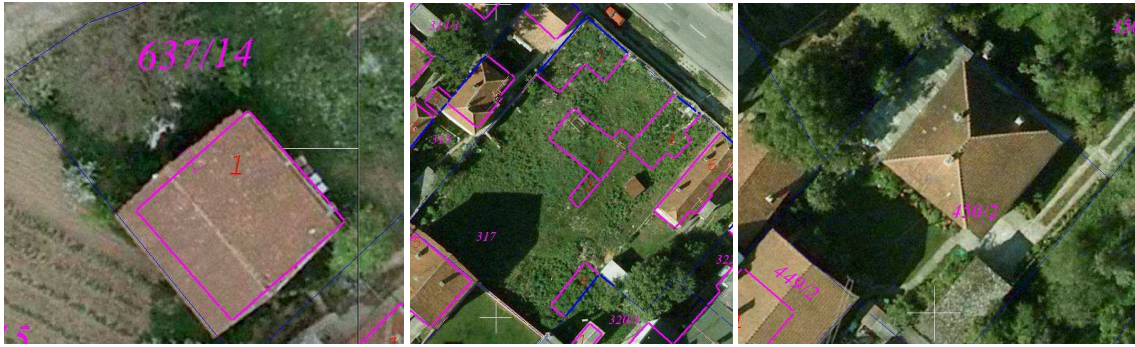
Figure 5: Mismatch between features on DCM (registered state) and DOP (real situation on the field) – position, shape and size of the building in DCM and DOP are in line (left); building does not exist in the field (demolished building) but it does exist in DCM (middle); building is established in the field but it does not exist in DCM (right)
