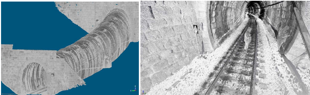
Figure 5 Raw point cloud of the rail tunnel.
