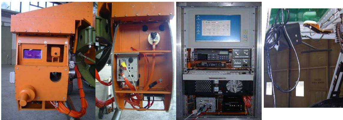
Figure 4: Appearance of one of the multi sensors (which is mounted on a helicopter) for synchronization and processing of geo spatial data, front side of sensor platform (rectangular window refers to part of the laser scanner Riegl LMS-Q560, large lens behind the device for calibration in the middle, it refers to IR camera, and small lens (up left) belongs to video camera (FGAN-FOM Research Institute for Optronics and Pattern Recognition, Ettlingen, Germany)
