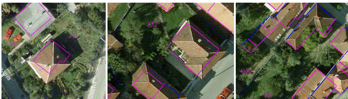
Figure 7: Errors on surveyed and mapped buildings – erroneously surveyed or mapped building on parcel (left); switched building line and auxiliary building line on parcel 352 (middle); switched building line and auxiliary building line on parcel 457 (right)
