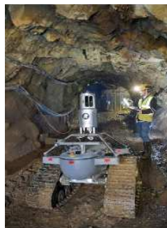
Figure 5: A robot with laser scanner owned by the company 3DMSI, for remote controlled recording
