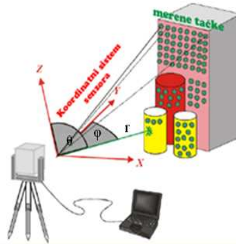
Figure 1: The principle of laser scanner operation
