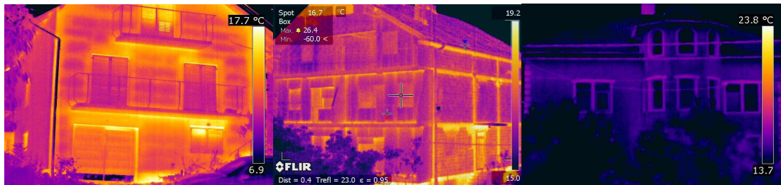
Figure 1: An example of survey of multi-storey building with thermovision sensors
