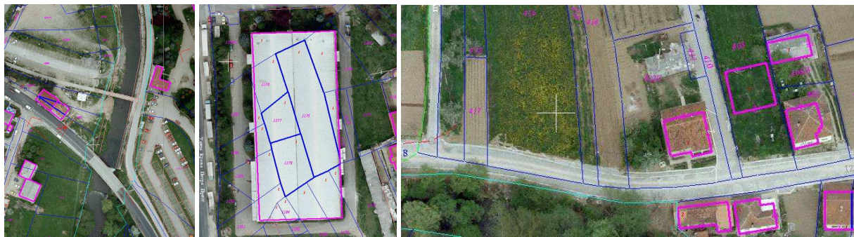
Figure 2: Mismatch between features on DCM (registered state) and DOP (real situation on the field) for CM Brus – regulation of Rasina riverbed (left); new building covers several parcels in DCM (middle); street reconstruction caused changes in parcel boundaries (right)
