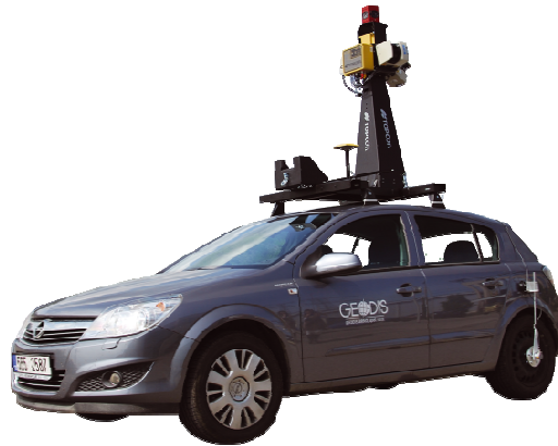
Fig. 1 Basic IP-S2 mobile mapping system configuration
