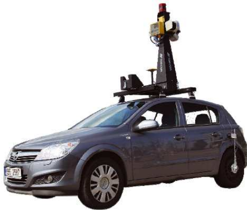
Figure 1: MMS on the road vehicle
