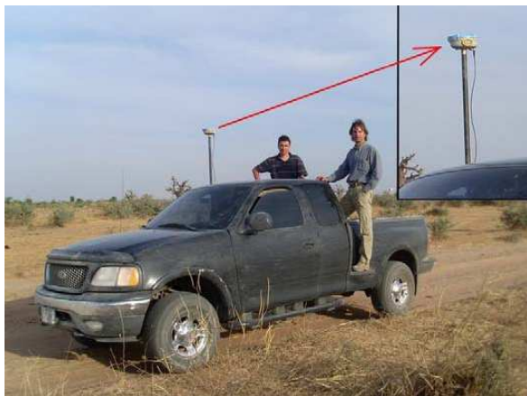
Picture 6: Vehicle with GPS receiver
