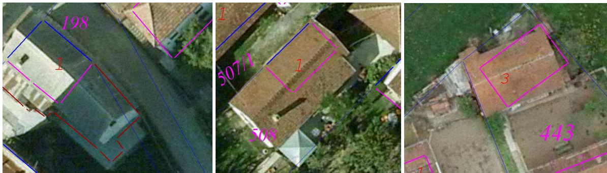
Figure 6: Mismatch between features on DCM (registered state) and DOP (real situation on the field) – part of the building exists in DOP, but not in DCM (left); building exists in DCM and DOP, but there is mismatch for their footprints due to the reconstruction of the building or demolition of old building and construction of new one (middle); building exists in DCM and DOP, but there is mismatch for their footprints due to the reconstruction of building or errors in survey of existing building (right)
