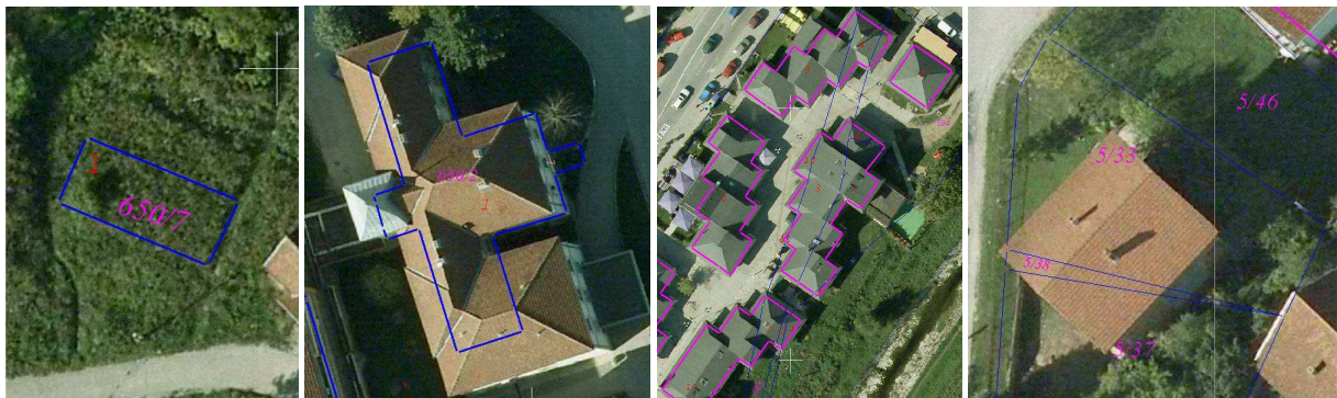
Figure 4: Mismatch between features on DCM (registered state) and DOP (real situation on the field) for CM Gornji Milanovac – parcel-building is established in the field, but it does not exist in DCM (left); parcel-building is recorded in DCM, but its size is wrong (second left); numerous buildings cover several parcels (second right); numerous newly constructed buildings cover several parcels (right)
