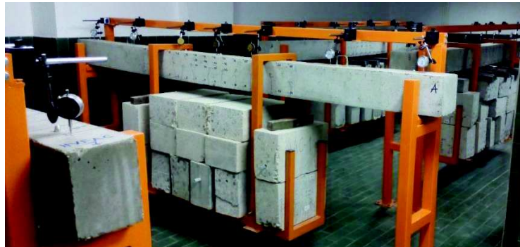
Figure 12 – NAC and RAC beams in the laboratory
