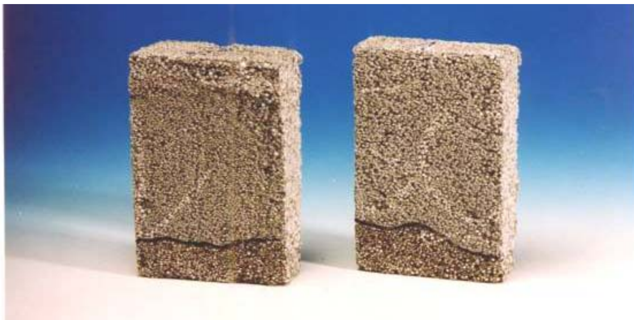
Slika 2. Visina upijanja vode nakon testa kapilarnog penjanja Figure 2. The height of absorbed water after capillary absorption test
