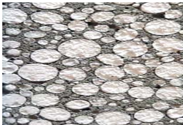
Slika 1. Struktura Simprolita Figure 1. The structure of Simprolit
