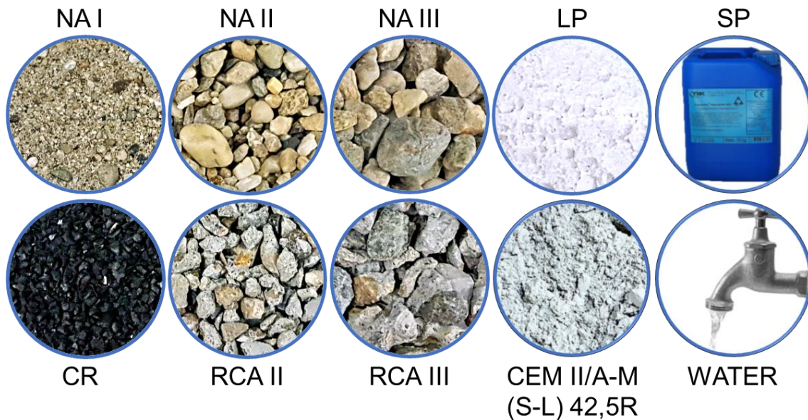
Figure 2: SCC components used in this research – natural aggregate fractions I, II and III (NA I, NA II, NA III), crumb rubber (CR) and recycled concrete aggregate fractions II and III (RCA II, RCA III), limestone powder (LP), portland-composite cement CEM II/A-M(S-L)42,5R, superplasticizer (SP) and water from the city water-works
