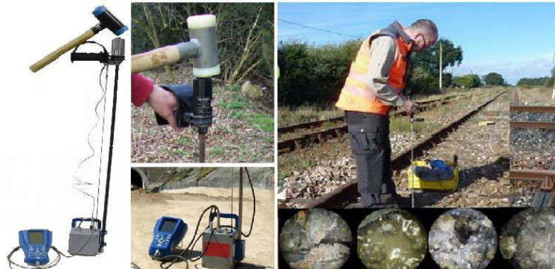
Figure 3. "PANDA" penetrometer ( http://www.macben.be/s9-draagkracht/?lang=en , 28.06.2017) and identification of track structure layers using endoscopy ( http://bsh-muc.com , 28.06.2017)
