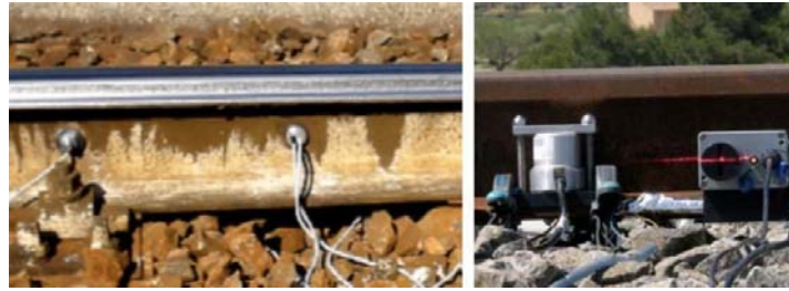
Figure 5. MPQY detector (left) (Molatefi and Mozafari, 2013) and mounted laser beam receiver and geophone (right) (INNOTRACK, 2006)
