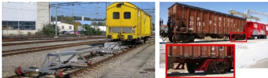
Figure 7. SBB vehicle for track stiffness measurements (left) (Nielsen et al., 2013; Wang et al., 2016) and mounting position of the UNL measurement system (right) (Wang et al., 2016)
