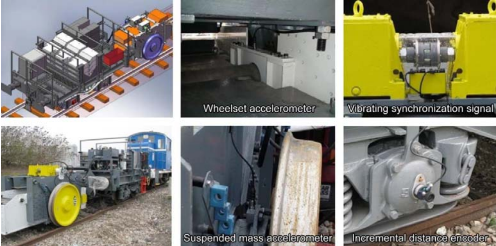
Figure 12. Schematic view and on-site measurement with Portancemètre (left) and sensors on the Portancemètre demonstrator (right) (Hosseingholian et al., 2011)
