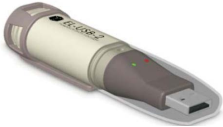
Figure 1. Data logger used for measuring air temperature and relative humidity
