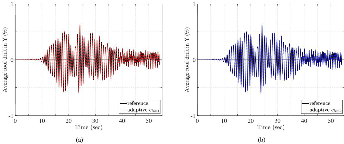
**Fig. 20.** Relative roof drift in Y under the Darfield ground acceleration for the non-adaptive section discretization with 108 MP and for two adaptive schemes with strain limits  $e_{lim,1}$  and  $e_{lim,2}$ .
