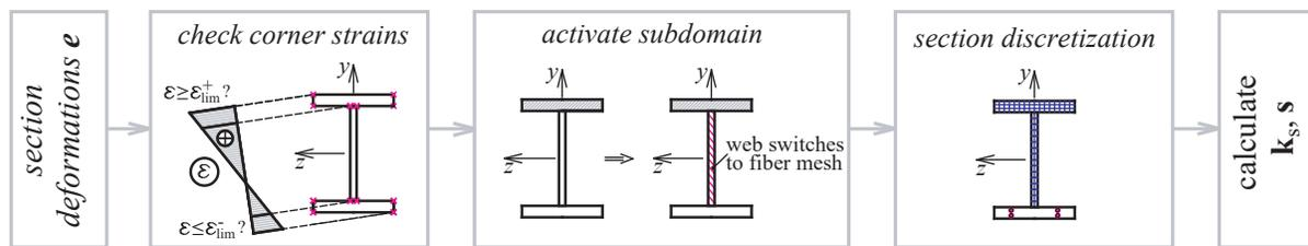
**Fig. 4.** Schematic outline of adaptive section discretization for a wide-flange section.
