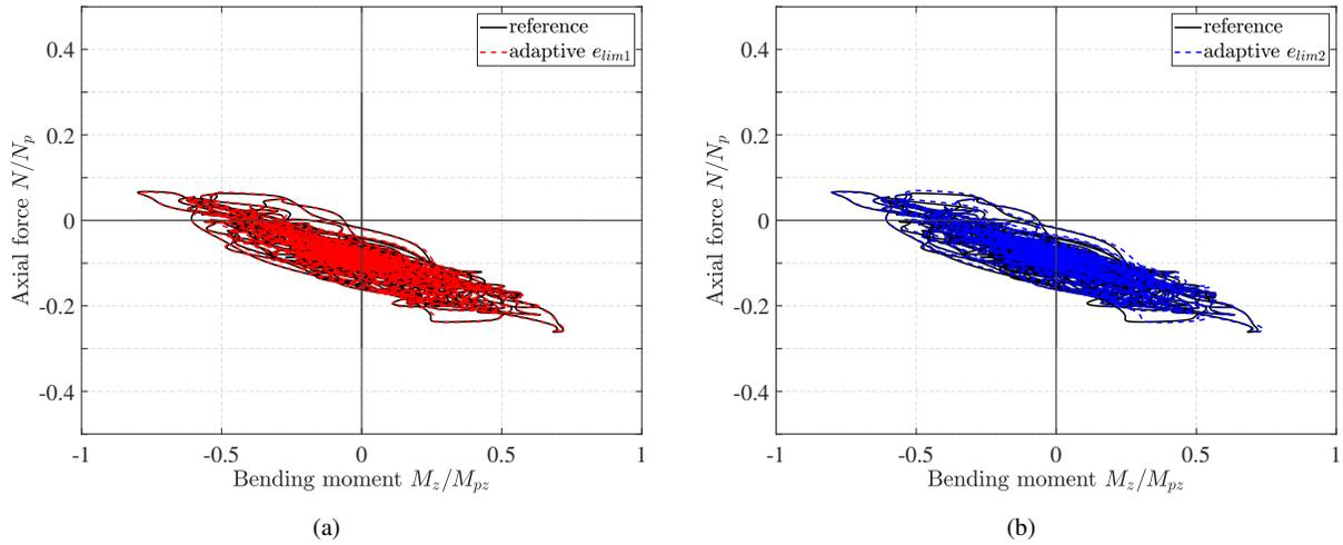
**Fig. 21.** Normalized axial force  $N$ -bending moment  $M_z$  history at the base of column 1 under the Darfield ground acceleration for the non-adaptive section discretization with 108 MP and for two adaptive schemes with strain limits  $e_{lim,1}$  and  $e_{lim,2}$ .
