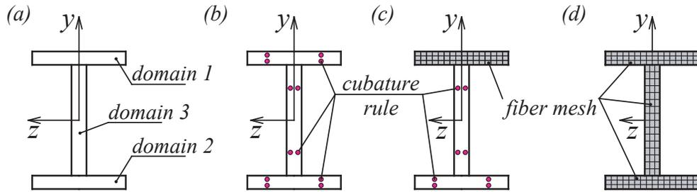
**Fig. 2.** Adaptive section discretization scheme for wide flange section: (a) division into 3 rectangular subdomains, (b) cubature rule for initial response, (c) fiber mesh for top flange after its activation, (d) section discretization after activation of all subdomains.
