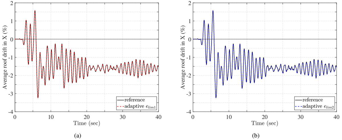
**Fig. 15.** Relative roof drift in X under the Kobe ground acceleration for the non-adaptive section discretization with 108 MP and for two adaptive schemes with strain limits  $e_{lim,1}$  and  $e_{lim,2}$ .
