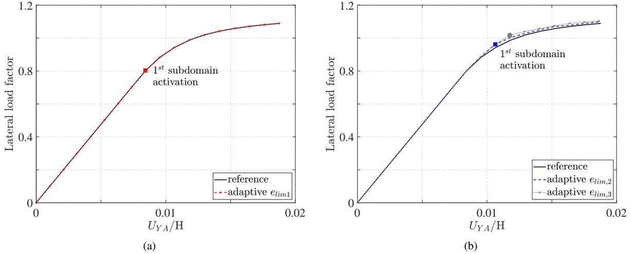
**Fig. 12.** Load-displacement response of 20-story frame for the non-adaptive section discretization with 108 MP and three adaptive schemes with strain limits  $e_{lim,1}$ ,  $e_{lim,2}$  and  $e_{lim,3}$
