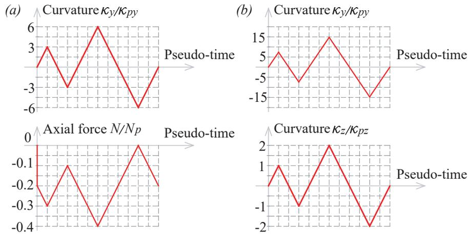
**Fig. 5.** Load history for section analyses: (a) curvature about y-axis with variable axial force, and (b) biaxial curvature under constant axial force  $N = (-0.20)N_p$
