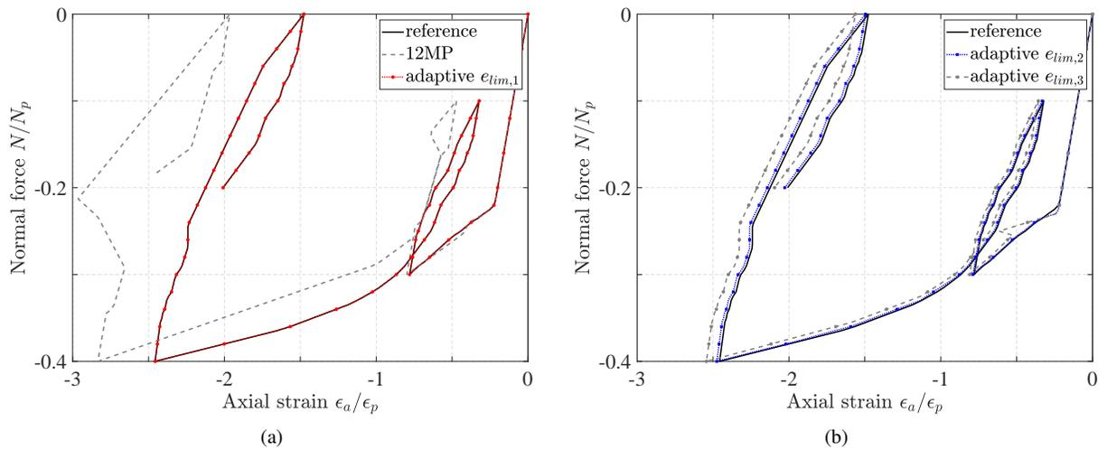
**Fig. 7.** Axial force-axial strain history for W14x120 steel section under variable axial force for two-non adaptive and 3 adaptive discretizations with strain limits  $e_{lim,1}$ ,  $e_{lim,2}$  and  $e_{lim,3}$ .
