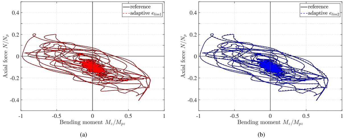
**Fig. 17.** Normalized axial force  $N$ -bending moment  $M_z$  history at the base of column 1 under the Kobe ground acceleration for the non-adaptive section discretization with 108 MP and for two adaptive schemes with strain limits  $e_{lim,1}$  and  $e_{lim,2}$
