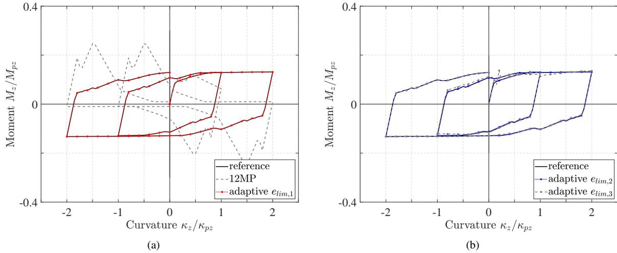
**Fig. 8.** Moment-curvature history about the  $z$ -axis for W14x120 steel section under constant axial force for two-non adaptive and 3 adaptive discretizations with strain limits  $e_{lim,1}$ ,  $e_{lim,2}$  and  $e_{lim,3}$ .
