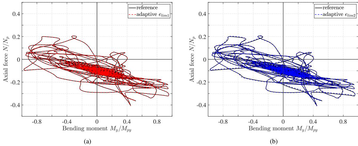
**Fig. 18.** Normalized axial force  $N$ -bending moment  $M_y$  history at the base of column 1 under the Kobe ground acceleration for the non-adaptive section discretization with 108 MP and for two adaptive schemes with strain limits  $e_{lim,1}$  and  $e_{lim,2}$ .
