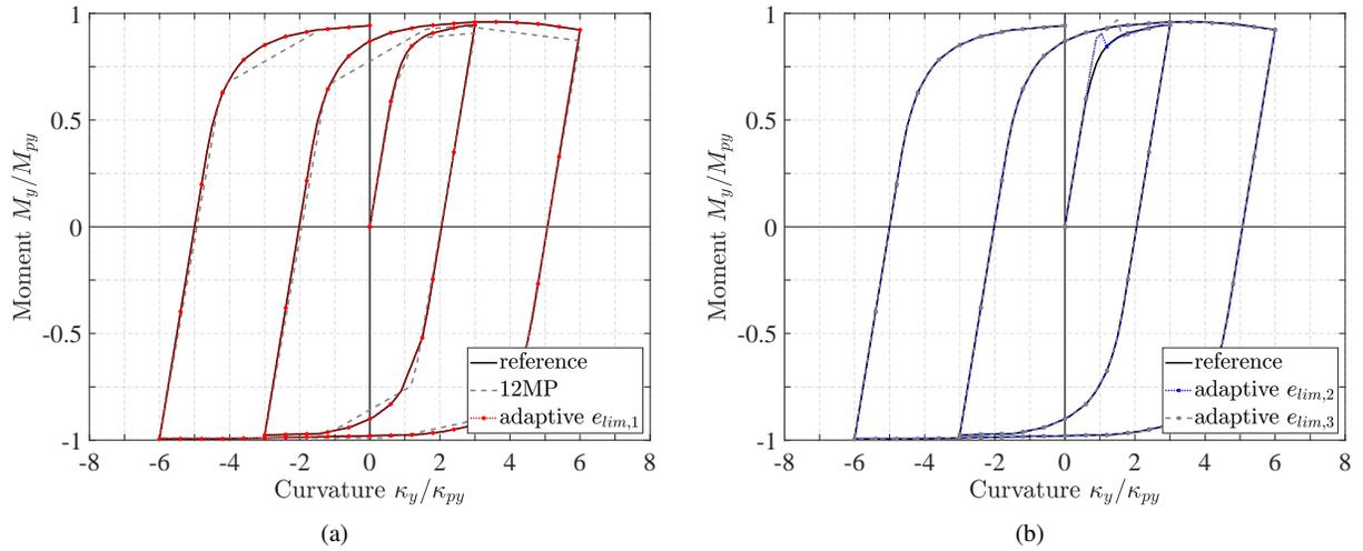
**Fig. 6.** Moment-curvature history for W14x120 steel section under variable axial force for two-non adaptive and 3 adaptive discretizations with strain limits  $e_{lim,1}$ ,  $e_{lim,2}$  and  $e_{lim,3}$ .
