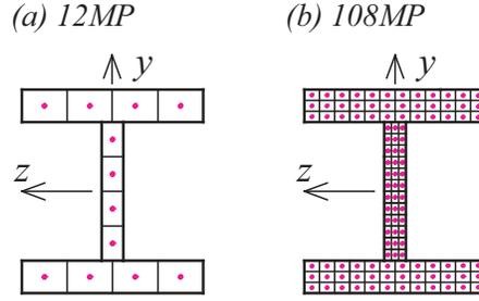
**Fig. 3.** Recommendations for wide flange section discretization with the midpoint integration rule from Kostic and Filippou (2012): (a) 12 MP scheme, (b) 108 MP scheme.
