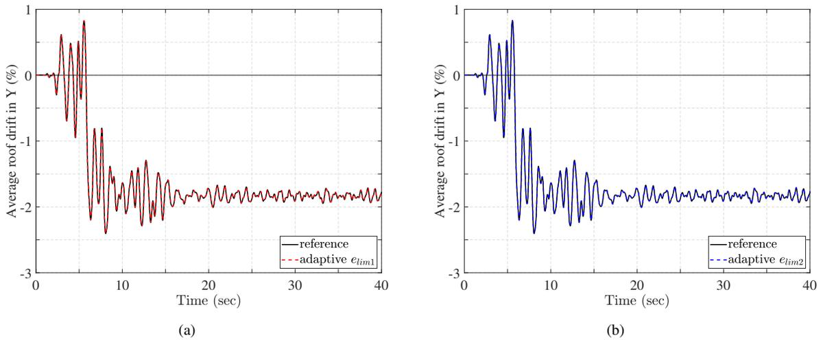
**Fig. 16.** Relative roof drift in Y under the Kobe ground acceleration for the non-adaptive section discretization with 108 MP and for two adaptive schemes with strain limits  $e_{lim,1}$  and  $e_{lim,2}$ .
