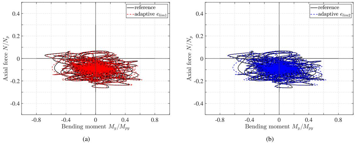
**Fig. 22.** Normalized axial force  $N$ -bending moment  $M_y$  history at the base of column 1 under the Darfield ground acceleration for the non-adaptive section discretization with 108 MP and for two adaptive schemes with strain limits  $e_{lim,1}$  and  $e_{lim,2}$ .
