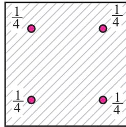
**Fig. 1.** Cubature rule for a unit square area with 4 IPs.
