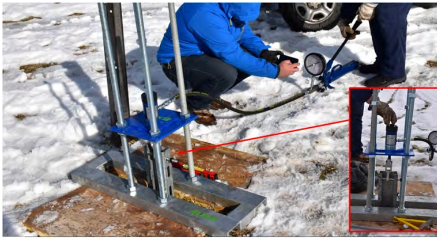
Figure 3: Modified extension kit for pull out tester
