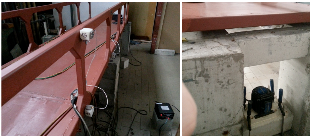
Figure 5. Accelerometer installed on the measured point of the model and shaker device to simulate ambient vibration installed over the support
