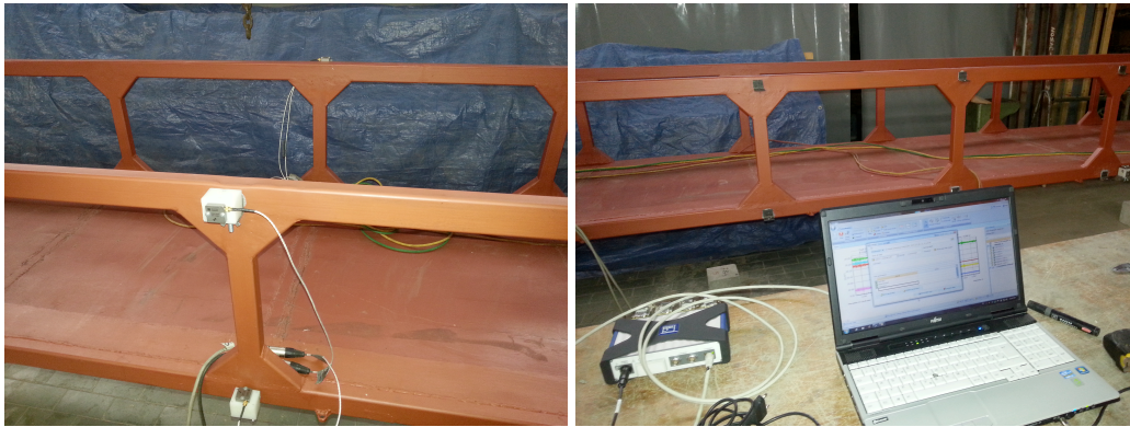
Figure 4. Positions of measurement points in one set with reference point for the model and acquisition system with laptop
