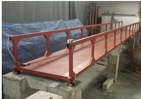
Figure 1. Tested Vierendeel bridge model structure in laboratory
