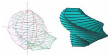
Fig. 7 Wireframe and solid model of spiral structure S4a (sphere/inscribed squares)
