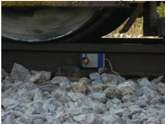
Fig.4. Position sensitive detector for sleeper vibration measurements
