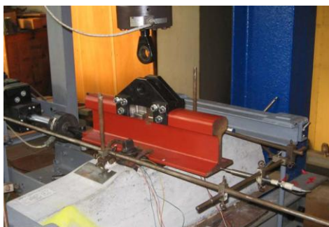
Fig.1. Test arrangement for determination of axial force during the longitudinal displacement of the rail [20]
