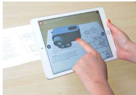
Figure 3: Combined overview of 3D model and its 2D images (technical drawings) in Augment application http://www.augment.com/portfolio-items/harran-university/
