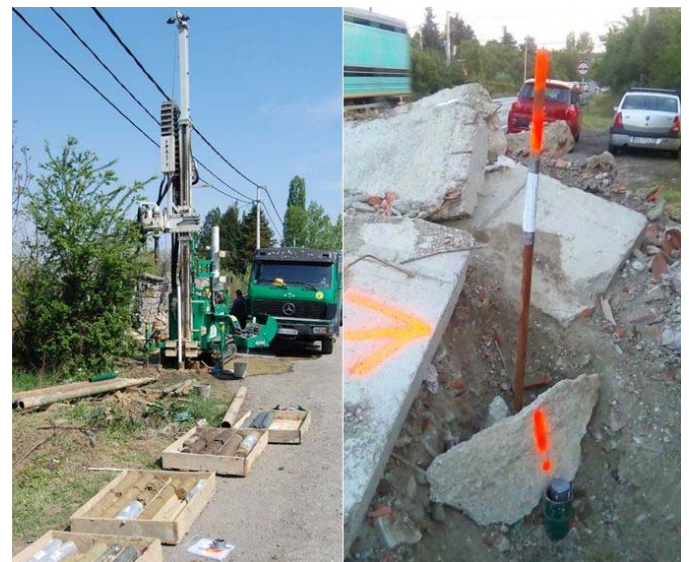
Figure 2 Borehole logging on the Umka landslide (left), destroyed inclinometer construction after 4 months from installation (right).
