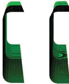
Figure 5 – Model without and with initial geometric imperfection
