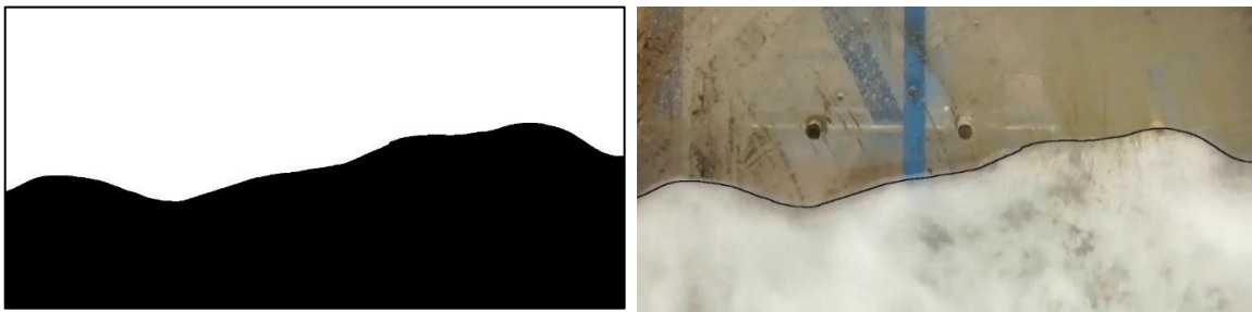
Figure 2. Left – Binarized image using global thresholding; Right – Original image with the FSI from contrast thresholding.
