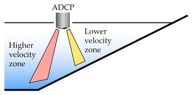
Figure 3. Signal interference near high-slope channel edges.
