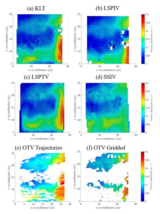
**Figure 4.** Gridded surface velocity maps for all algorithms, including the original trajectory map for OTV (**e**).
