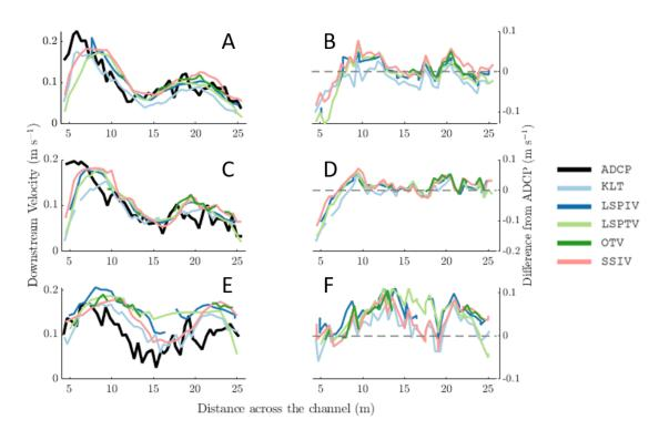
**Figure 9.** Cross-sectional analysis of Video B processed with all algorithms against the ADCP data. The left panels represent three different cross-sections ((A = S1, C = S2, and E = S3), the right panels represent the difference from the ADCP of the three cross-sections (B = S1, D = S2, and F = S3). The distance across the channel relates to the y co-ordinates in Figures 2, 4 and 6. 5 m is the right bank, and 25 m is the left bank.
