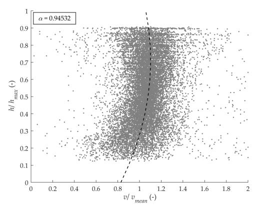
**Figure 5.** ADCP relative velocity magnitude data. Characteristic velocity profile obtained using second-degree polynomial fit. The alpha value represents the ratio between the extrapolated surface velocity and the depth-averaged velocity.
