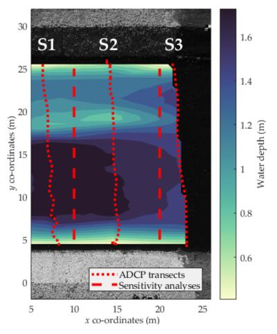
**Figure 2.** Bathymetry profile of the Region of Interest, including the locations of ADCP transects (from left to right: S1, S2 and S3), and sensitivity analysis transects (from left to right cross-section 10 m and 20 m).
