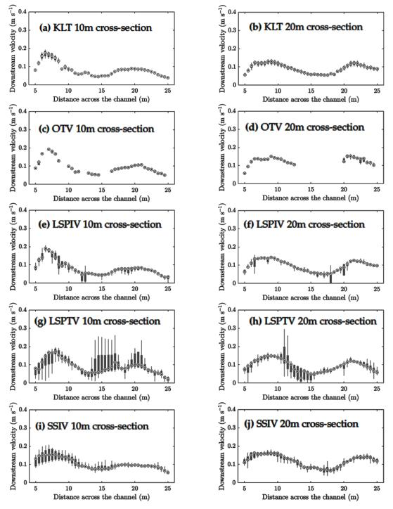
**Figure 7.** Sensitivity Analysis results for all algorithms at two cross-sections (Represented by red dashed lines in Figure 2). The distance across the channel relates to the y co-ordinates in Figures 2, 4 and 6. 5 m is the right bank, and 25 m is the left bank.
