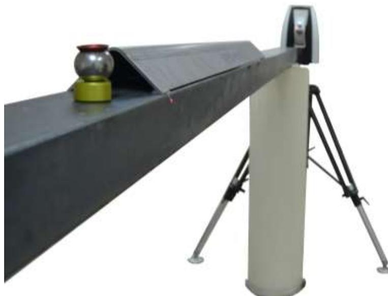
**Fig. 2.** Laser tracker setup with installed specimen.
