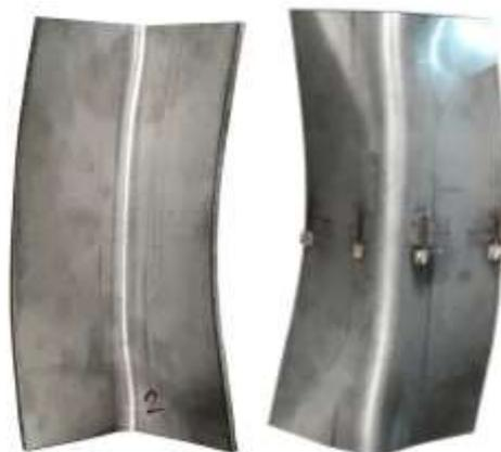
**Fig. 7.** Stub column failure mode of specimen ACF  $80 \times 80 \times 4 - 240 - 2$ .
