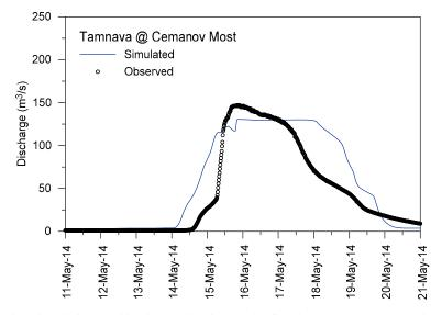
**Figure S3.** Simulated and observed hydrographs during the flood event in May 2014: the Ćemanov Most stream gauge at the Tamnava River.
