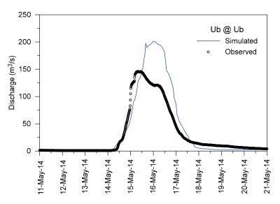
Figure S4. Simulated and observed hydrographs during the flood event in May 2014: the Ub stream gauge at the Ub River.
