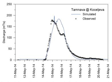
Figure S2. Simulated and observed hydrographs during the flood event in May 2014: the Koceljeva stream gauge at the Tamnava River.
