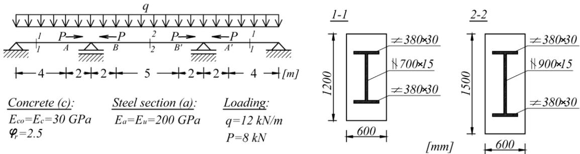
Fig. 1. Continuous composite beam
