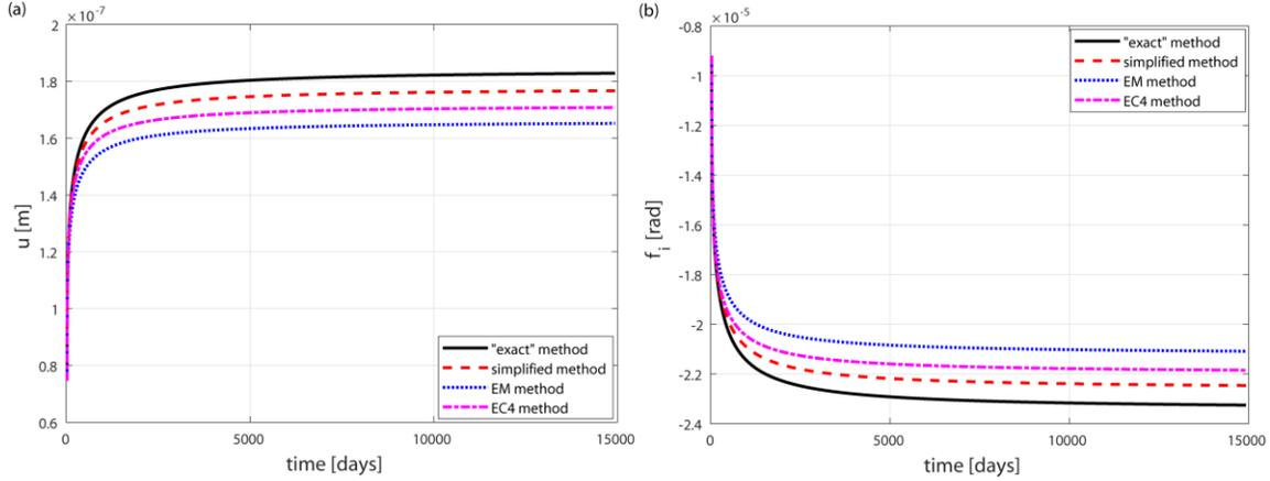
Fig. 3. Comparison of generalized displacements  $u$  and  $\varphi$  over time for four analysis methods
