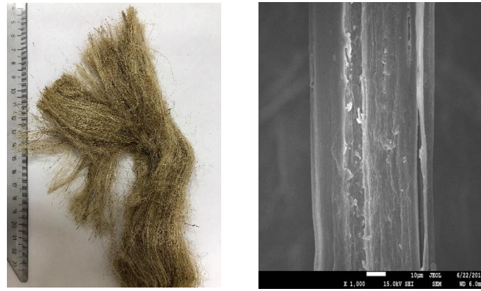
Figure 2. Bundle of hemp fibres (left) and hemp fibre image under a scanning electron microscope (right)
