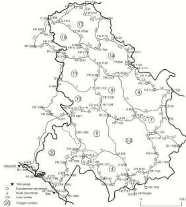
Figure 5. High accuracy leveling network
