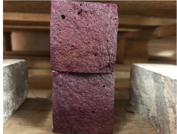
Figure 10. Appearance of the sample surface after treatment with phenolphthalein solution test
