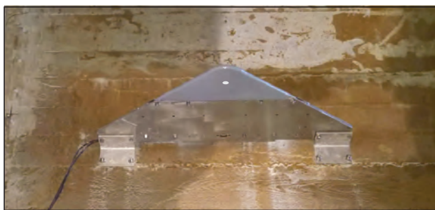
Figure 6. Different types of EM probes: 1D LOG-type for fixed installation in large tunnels
