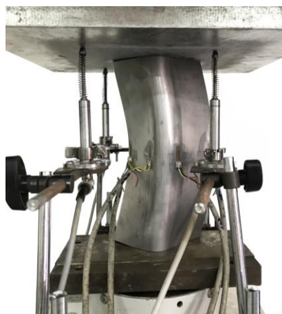
Figure 2 - Typical stub column failure mode [1]
