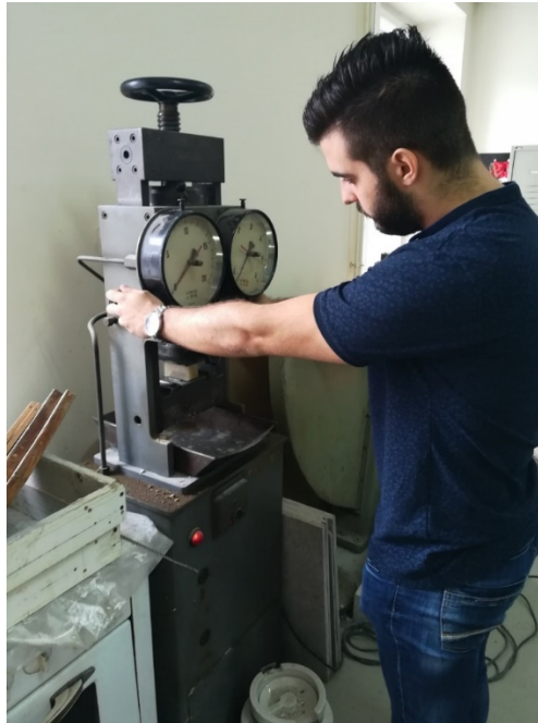
Figure 3. Compressive strength test using Amsler hydraulic press
