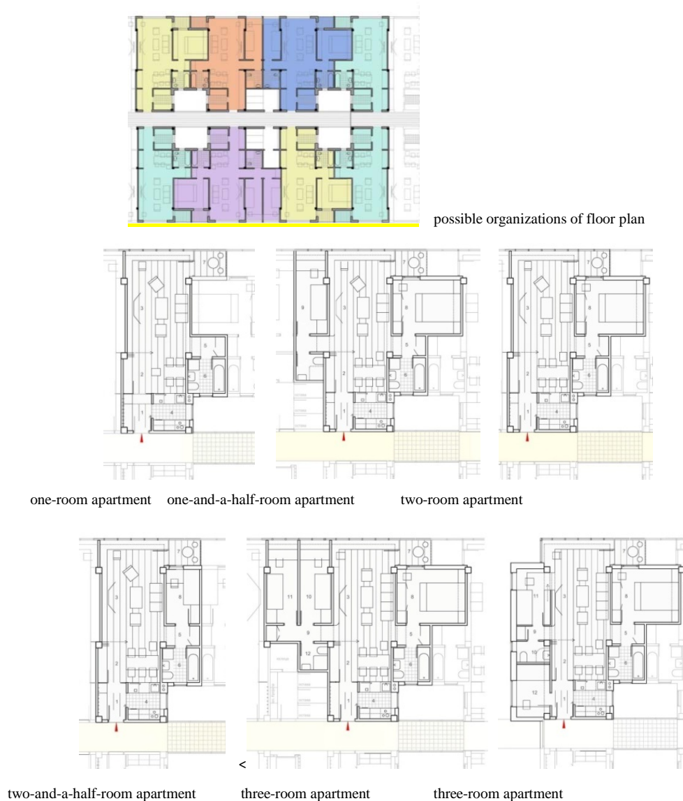
Figure 4. Flexibility of internal space - Proposition for social housing Dr. Ivan Ribar Belgrade /Marušić D, Marušić M. (2011) Belgrade, Serbia 4
