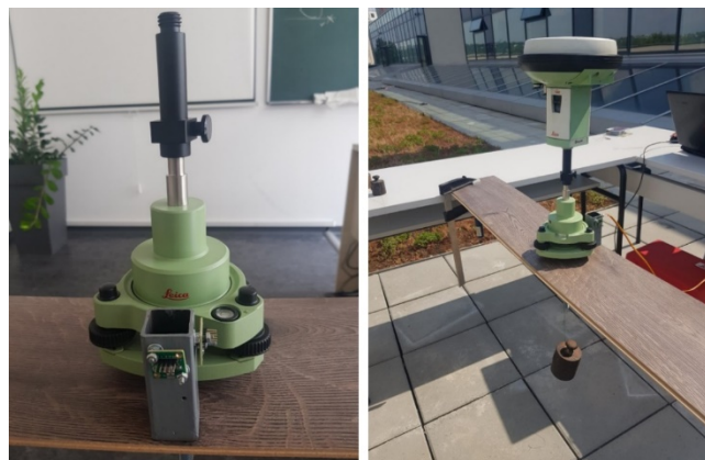
Figure 3. Accelerometer, tribrach and GNSS receiver carrier (a), construction with beam and sensors (b)
