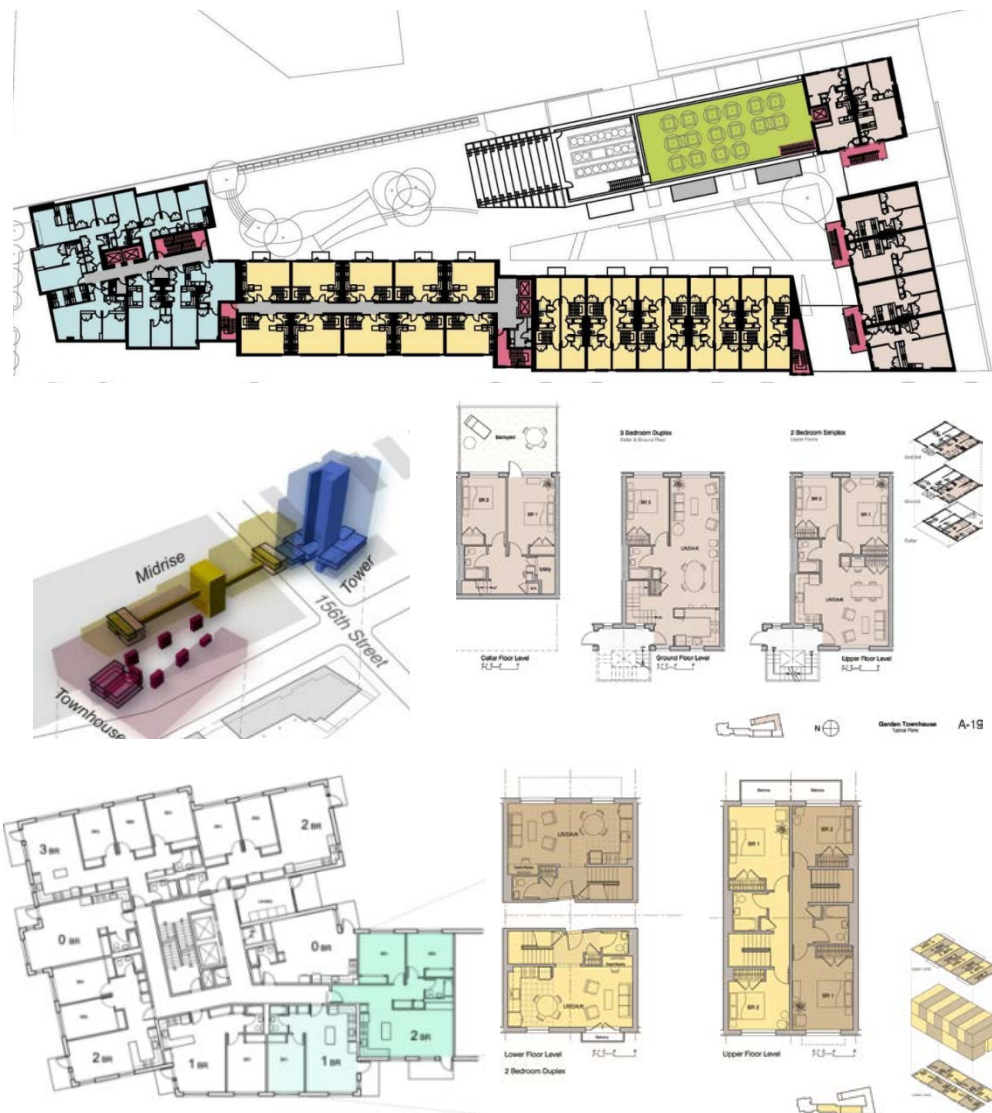
Figure 3. Distribution of different apartment units' types Via Verde / Grimshaw & Dattner Architects (2012), New York, USA 3
