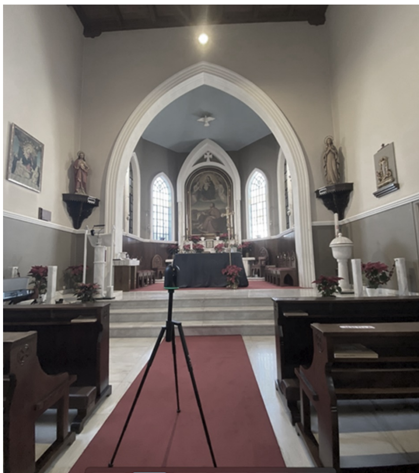
Figure 12. Laser scanning process for capturing the church structure from inside [Authors]
