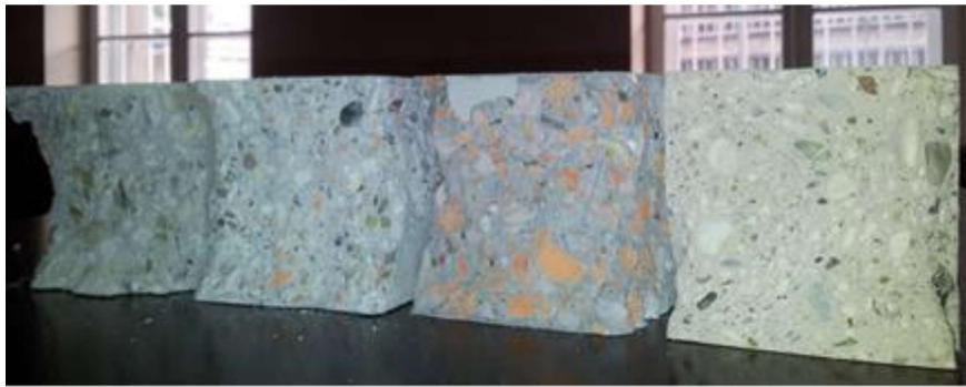
Figure 3. The appearance of the fracture surface of the concrete with different content of recycled brick aggregate
