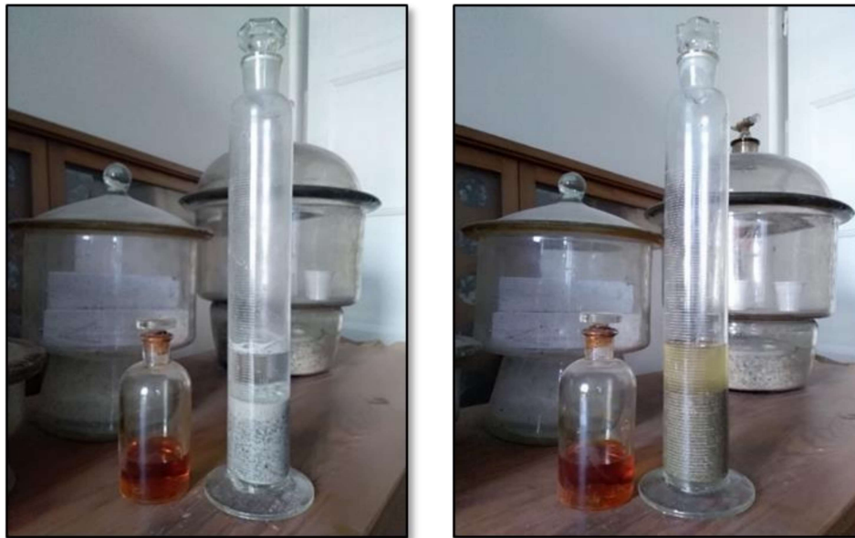
Figure 4. Organic content testing of fine aggregates – transparent solution for recycled (left) and colored for river (right) aggregate
