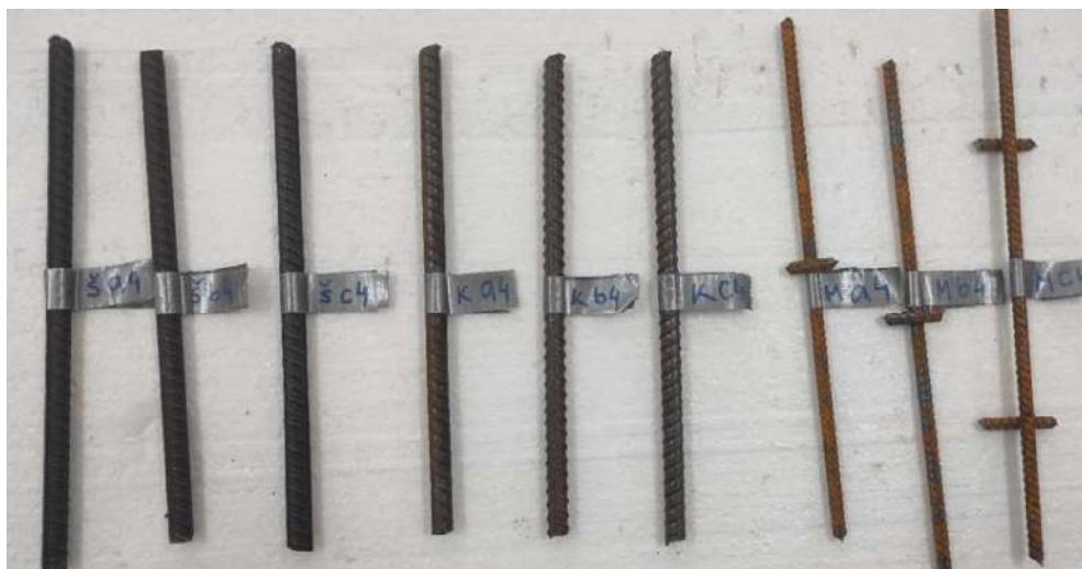
Figure 5. Samples of bars, coils and welded fabrics that were prepared for the ageing at the temperature of 100°C in duration of 2 h
