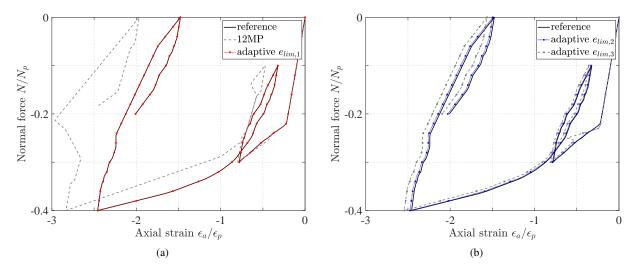
**Fig. 7.** Axial force-axial strain history for W14x120 steel section under variable axial force for two-non adaptive and 3 adaptive discretizations with strain limits  $e_{lim,1}$ ,  $e_{lim,2}$  and  $e_{lim,3}$ .
