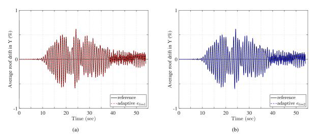
**Fig. 20.** Relative roof drift in Y under the Darfield ground acceleration for the non-adaptive section discretization with 108 MP and for two adaptive schemes with strain limits  $e_{lim,1}$  and  $e_{lim,2}$ .
