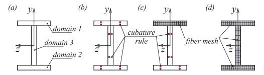
**Fig. 2.** Adaptive section discretization scheme for wide flange section: (a) division into 3 rectangular subdomains, (b) cubature rule for initial response, (c) fiber mesh for top flange after its activation, (d) section discretization after activation of all subdomains.
