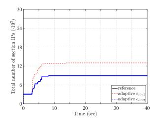
**Fig. 14.** Evolution of the total number of section integration points (IPs) under the Kobe acceleration record for the non-adaptive section discretization with 108 MP and for two adaptive schemes with strain limits  $e_{lim,1}$  and  $e_{lim,2}$ .
