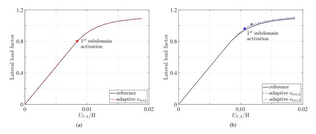
**Fig. 12.** Load-displacement response of 20-story frame for the non-adaptive section discretization with 108 MP and three adaptive schemes with strain limits  $e_{lim,1}$ ,  $e_{lim,2}$  and  $e_{lim,3}$
