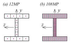
**Fig. 3.** Recommendations for wide flange section discretization with the midpoint integration rule from Kostic and Filippou (2012): (a) 12 MP scheme, (b) 108 MP scheme.
