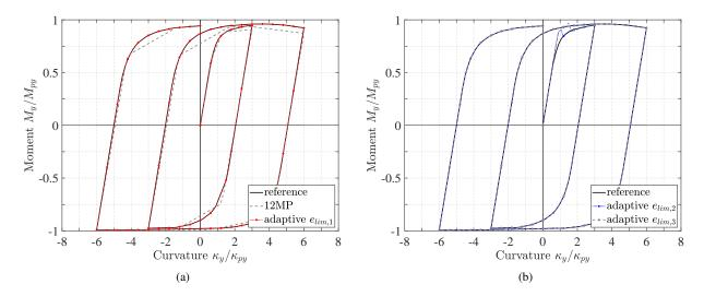
**Fig. 6.** Moment-curvature history for W14x120 steel section under variable axial force for two-non adaptive and 3 adaptive discretizations with strain limits  $e_{lim,1}$ ,  $e_{lim,2}$  and  $e_{lim,3}$ .
