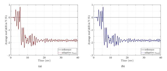
Fig. 16. Relative roof drift in Y under the Kobe ground acceleration for the non-adaptive section discretization with 108 MP and for two adaptive schemes with strain limits  $e_{lim,1}$  and  $e_{lim,2}$ .
