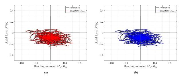
**Fig. 22.** Normalized axial force *N*-bending moment  $M_y$  history at the base of column 1 under the Darfield ground acceleration for the non-adaptive section discretization with 108 MP and for two adaptive schemes with strain limits  $e_{lim,1}$  and  $e_{lim,2}$ .
