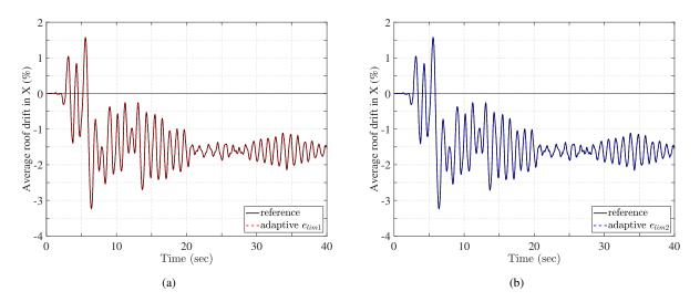
Fig. 15. Relative roof drift in X under the Kobe ground acceleration for the non-adaptive section discretization with 108 MP and for two adaptive schemes with strain limits  $e_{lim,1}$  and  $e_{lim,2}$ .
