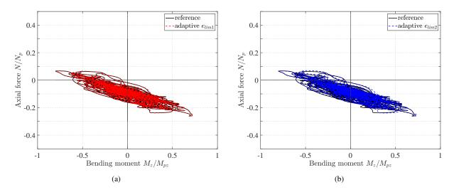
Fig. 21. Normalized axial force N-bending moment  $M_z$  history at the base of column 1 under the Darfield ground acceleration for the non-adaptive section discretization with 108 MP and for two adaptive schemes with strain limits  $e_{lim,1}$  and  $e_{lim,2}$ .
