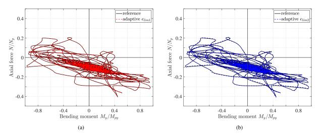
**Fig. 18.** Normalized axial force *N*-bending moment  $M_y$  history at the base of column 1 under the Kobe ground acceleration for the non-adaptive section discretization with 108 MP and for two adaptive schemes with strain limits  $e_{lim,1}$  and  $e_{lim,2}$ .
