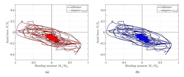
Fig. 17. Normalized axial force *N*-bending moment  $M_z$  history at the base of column 1 under the Kobe ground acceleration for the non-adaptive section discretization with 108 MP and for two adaptive schemes with strain limits  $e_{lim,1}$  and  $e_{lim,2}$
