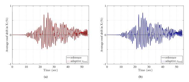
**Fig. 19.** Relative roof drift in X under the Darfield ground acceleration for the non-adaptive section discretization with 108 MP and for two adaptive schemes with strain limits  $e_{lim,1}$  and  $e_{lim,2}$ .
