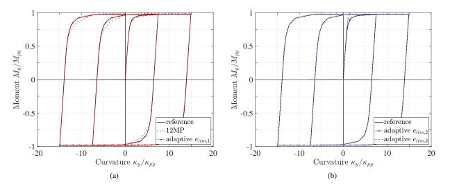
**Fig. 9.** Moment-curvature history about the *y*-axis for W14x120 steel section under constant axial force for two-non adaptive and 3 adaptive discretizations with strain limits  $e_{lim,1}$ ,  $e_{lim,2}$  and  $e_{lim,3}$ .
