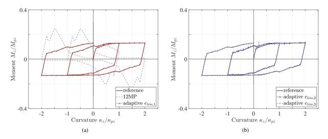
**Fig. 8.** Moment-curvature history about the *z*-axis for W14x120 steel section under constant axial force for two-non adaptive and 3 adaptive discretizations with strain limits  $e_{lim,1}$ ,  $e_{lim,2}$  and  $e_{lim,3}$ .
