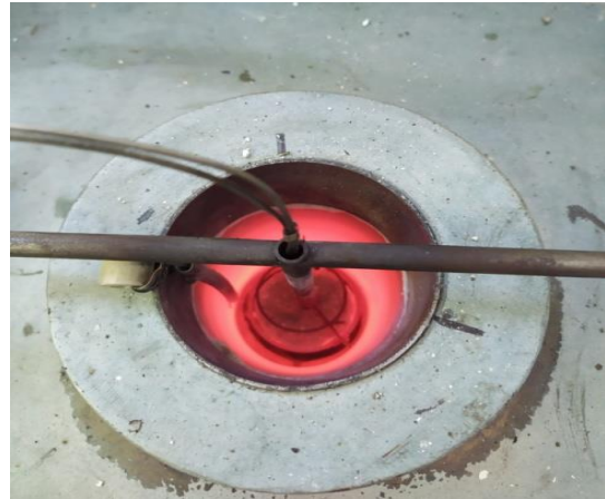
Fig. 3. The standard furnace for non-combustibility test
