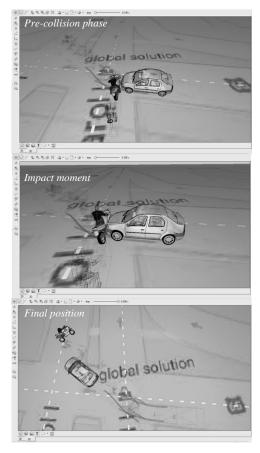
Fig.18 Collision phases identification.
