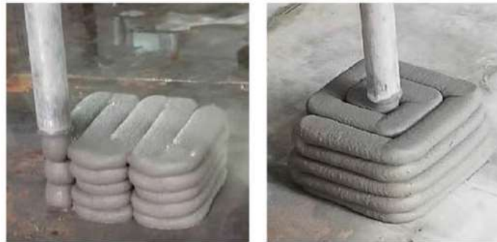
Fig. 1. FDM technology for 3D printing of concrete. [7]
