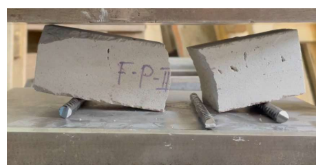
Fig. 13. Fracture of sample in compressive strength test Fig. 14. Fracture of sample in flexural strength test
