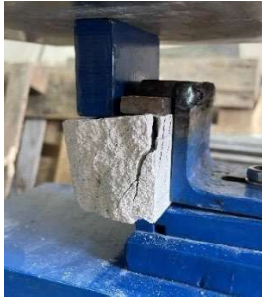
Fig. 10. Fracture of samples from series 1 in shear test
