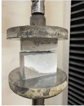
Fig. 15. Fracture of sample from series 1 in axial tension test
