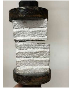
Fig. 16. Fracture of sample from series 2 in axial tension test
