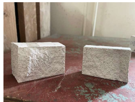
Fig. 18. The segments of the samples after reaching the ultimate load
