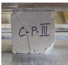
Fig. 13. Fracture of sample in compressive strength test Fig. 14. Fracture of sample in flexural strength test
