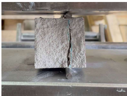
Fig. 17. Fracture of sample in splitting test
