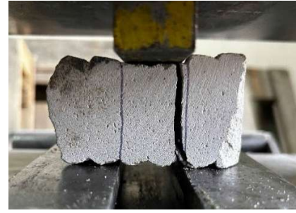
Fig. 11. Fracture of samples from series 2 in shear test
