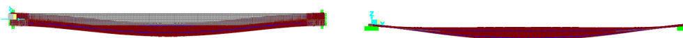
Figure 6. First lateral-torsional mode shape of the bridge: top view (left), side view (right)
