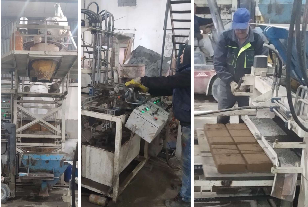
Fig 3. The process of making porous concrete slabs
