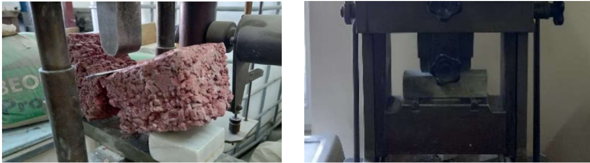
Fig. 3 Three-point flexural strength test
