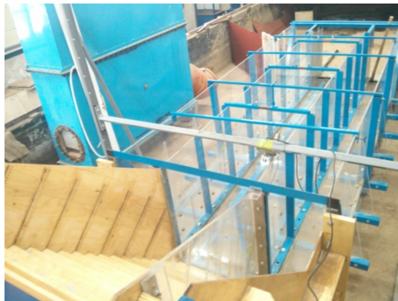
Figure 3. Scale model of converging stepped chute with stilling basin.
