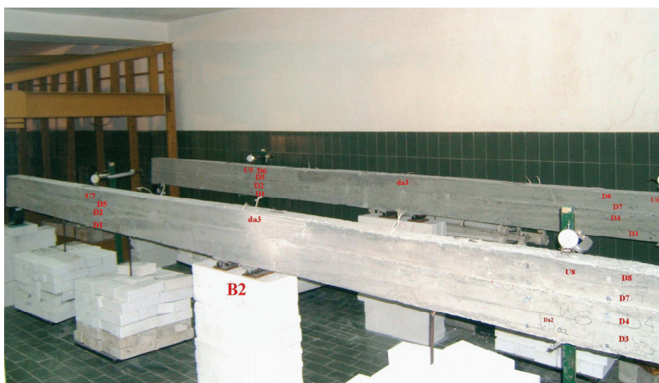
Fig. 2. Girders B1 and B2 with measurement points
