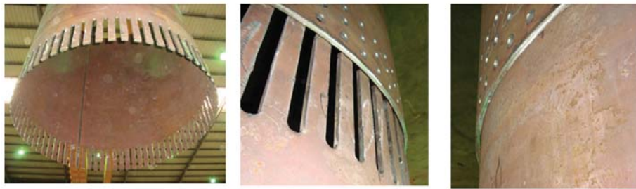
Figure 3. Main concept of the friction connection in tubular tower for wind turbines
