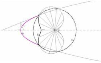
Figure 4: Harmonic equivalent of the parabolic cylinder – the surface of the 4<sup>th</sup> order with a spike
