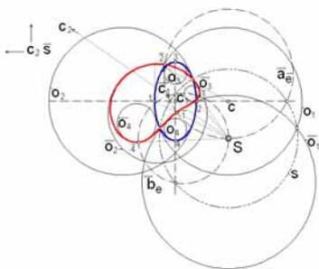
Figure 7: Ellipse and the 4<sup>th</sup> order curve with two circular axes of harmonic symmetry - bean curve
