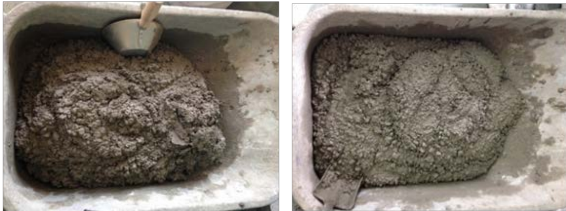
Figure 4.147 a) HVFAC mixture C200_F200 b) OPCC mixture OPC_S
