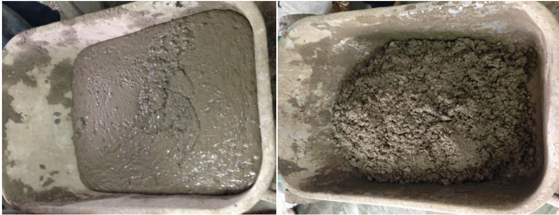
Figure 4.8 a) HVFAC mixture C200_F350 b) OPCC mixture OPC_F
