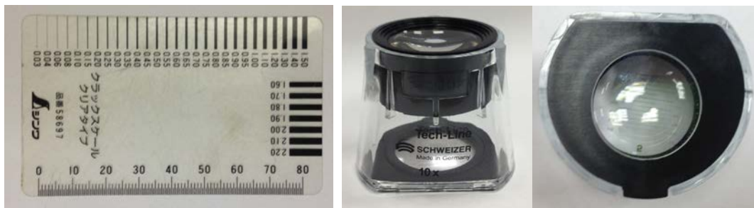
Figure 4.24 a) Crack width comparator, b) magnifying glass (10x)
