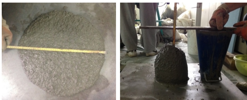
Figure 4.28 Slump/flow measurements of mixtures a) C200_F350 and b) OPC_F
