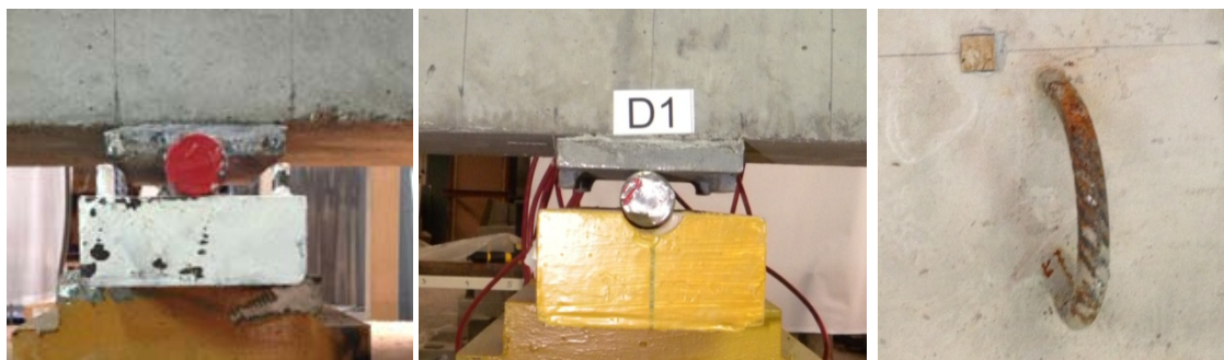
Figure 4. 13 The beams: a) free support b) fixed support, and c) steel hook
