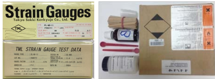
Figure 4.23 a) Strain gauge test data and b) HBM glue for strain gauges
