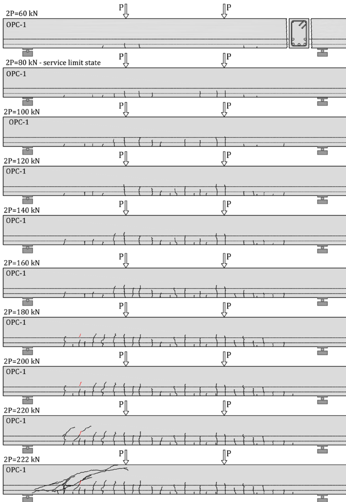
Figure 4.245 Crack patterns on the OPC-1 beam
