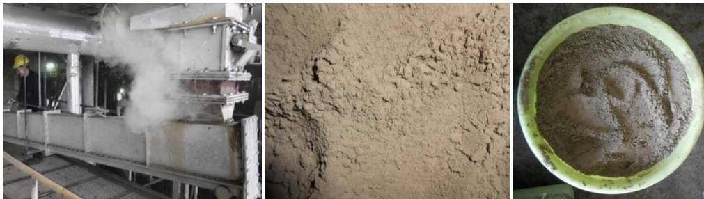
Figure 4.1 a) Sampling location in "Nikola Tesla B" power plant, b, c) FA sample
