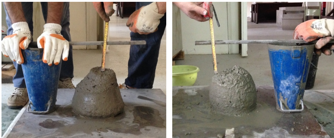
Figure 4.160 Slump measurements of a) C200_F200 and b) OPC_S concrete mixtures
