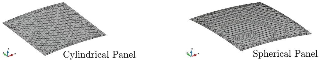
Figure 10.51: Unstructured meshes of triangular layered finite elements
