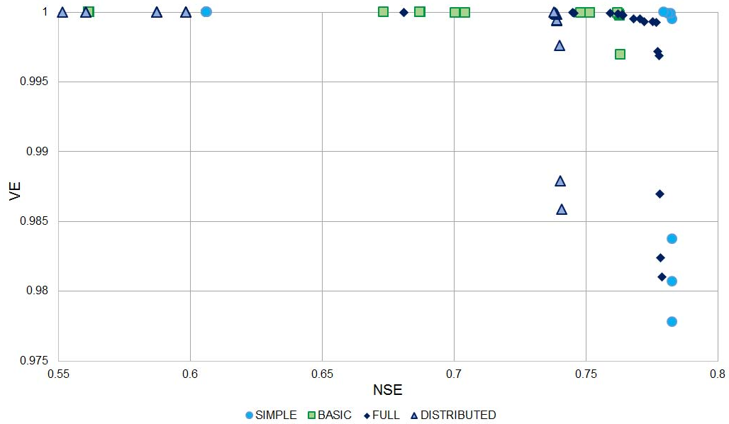
Figure 112. Pareto fronts of the SIMPLE, BASIC, FULL and distributed versions of the model obtained by calibration in 2007-2012 for the Toplica River catchment.
