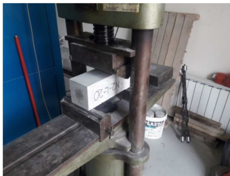
Figure 5 – Three point bending test
