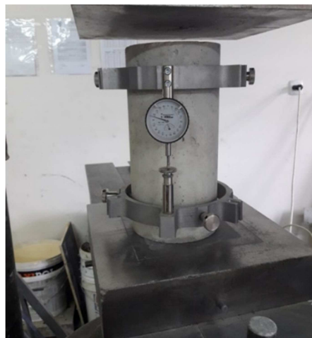
Figure 7 – Measuring of modulus of elasticity
