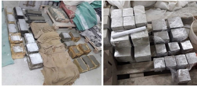
Figure 2 – Sample treatment after casting (left) and C-samples treatment after demoulding (right)
