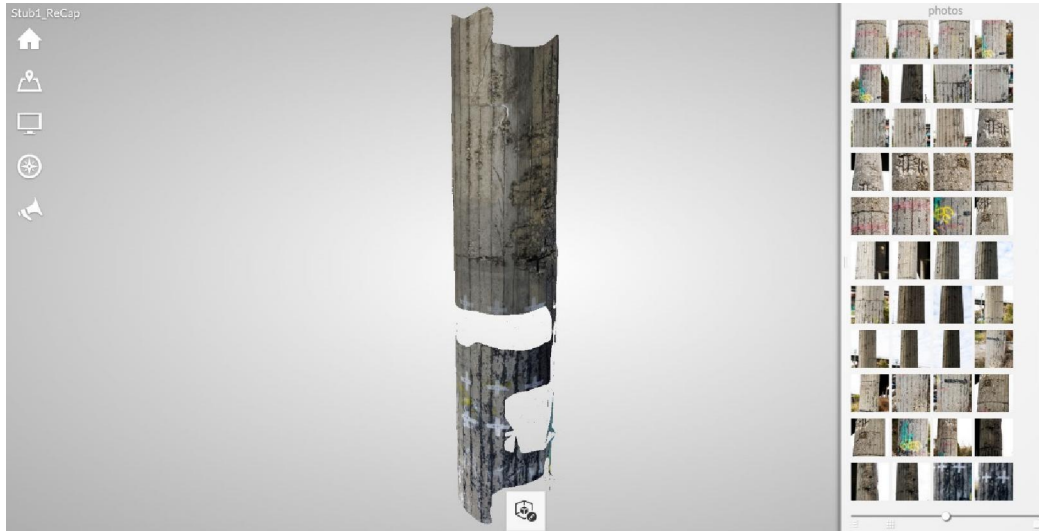
Figure 4.9. Concrete column reality mesh generated by Autodesk ReCap.
