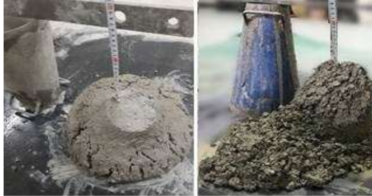
Figure 11. Possible forms of slump (true slump - left, shear slump - right)
