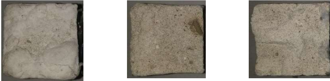
Figure 4 – Samples exposed to solution of sodium-chloride before and after the test
