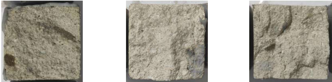
Figure 4 – Samples exposed to solution of sodium-chloride before and after the test
