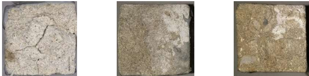
Figure 5 – Samples exposed to solution of sodium-sulfate before and after the test
