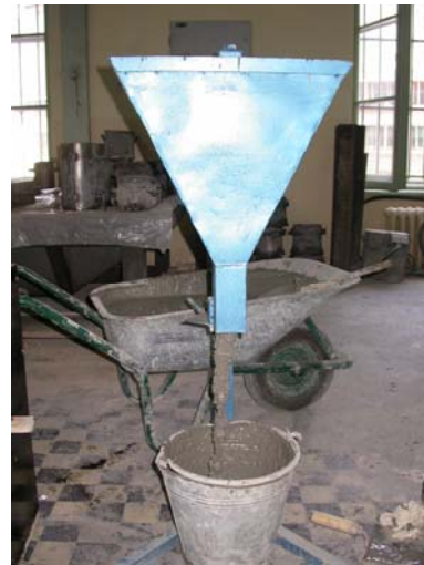
Figure 3. T500 test – time until fresh concrete reaches diameter of 500 mm is measured (left) and V-funnel test where the time needed for all of the concrete to fall out of funnel (right) is measured
