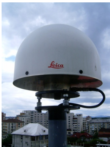
Slika 7.1.8 – Antena LEIAT504 na krovu NACLR (National Agency for Cadastre and Land Registration) zgrade u Baja Mareu (izvor: http://www.epncb.oma.be/networkdata/siteinfo4onestation.php?station=BAIA00ROU )
