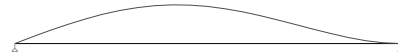
Figure 5a. The first mode shape for the tube, simple supported at one end and fixed at the second, f_{01}=1.70\text{Hz}
